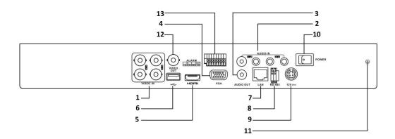
The rear panel of DS-7208HUHI-F2/N and DS-7216HUHI-F2/N provides 8 and 16 video input interfaces respectively.
